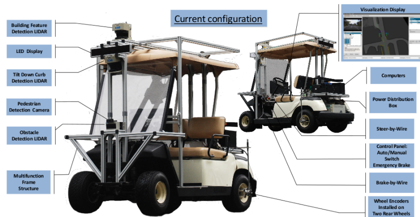
Fig. 3: Autonomous vehicle hardware architecture.
