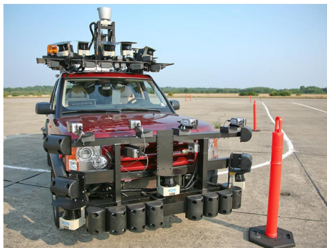
Fig. 2. The MIT’s vehicle at the Darpa Urban Challenge.
