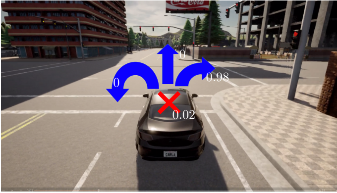
Figure 9.11: Output policy for vehicle at s = (2, 0, \text{west}, 2, 0, L) (or at t = 1 in Figure 9.10). The straight action would result in a violation of specification \varphi_G while taking right leads to a path like that in Figure 9.10b.
